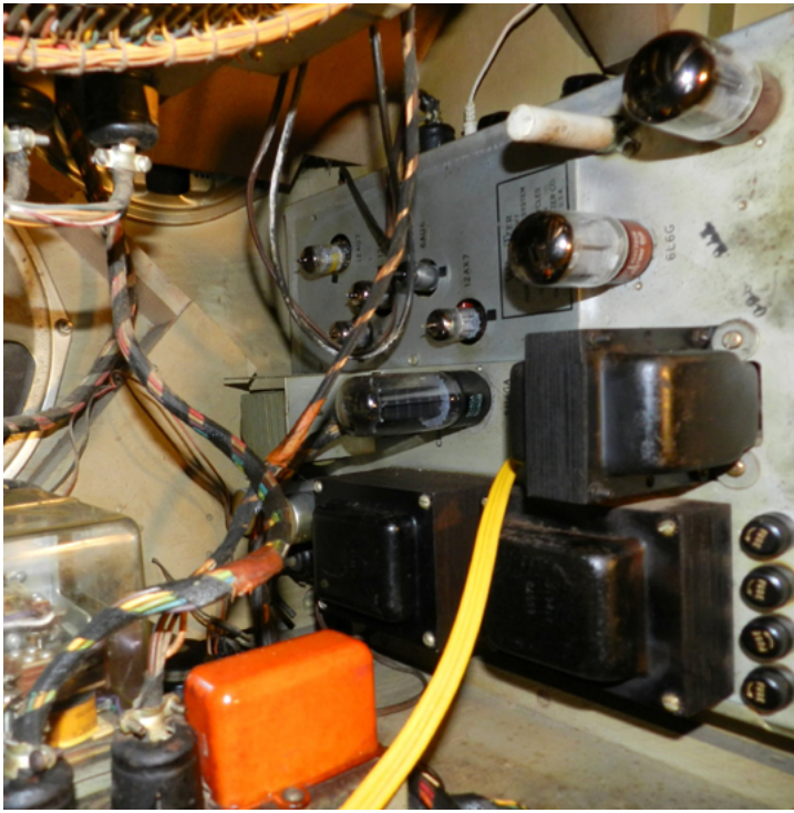
Wurlitzer 530 amp back into place inside the 'Centennial 2000'. (KB8TAD photo)
