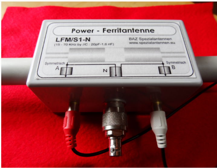
BAZ VLF S1-N 15-70 kHz receiver. (Courtesy of the author)
