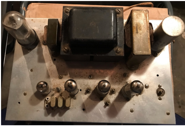
A recent hamfest find in this beautifully built homebrew AM transmitter for 2 meters. The seller said he did not know what it was. My older and more experienced eyes had a hunch and the 36 MHz crystals confirmed by suspicions. The top needs some cleaning, but a look at the underside reveals the excellent workmanship that went into the build and serves as a quick trip back in time concerning the parts used – popular in their day. (WA3UVV photo)
