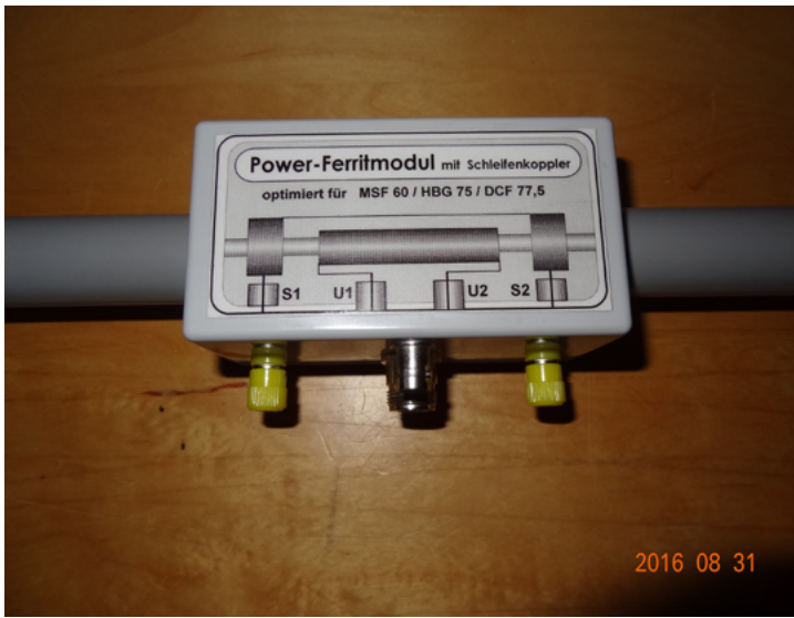
BAZ power ferrite module for SFTS stations. (Courtesy of the author)
