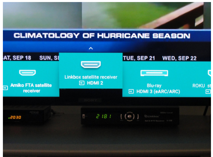
Sony Bravia TV lets users customize HDMI port labels. All four of available HDMI ports are labelled for the various inputs. (KS4ZR photo)
