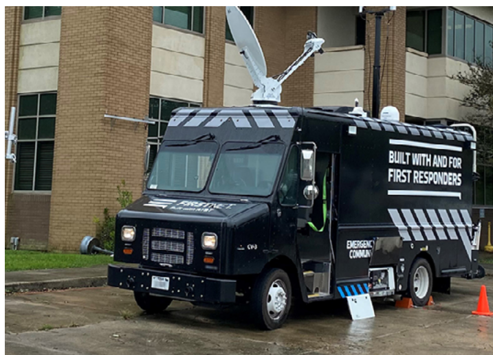
Another of AT&T's 76 mobile communications assets (this one sporting a Ku-band antenna) that can quickly be deployed to major storm sites. (Courtesy: AT&T)
